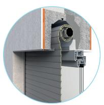
In this case, roller shutters are installed in special lintels. It is a very clean and elegant solution where the roller shutter system becomes a part of the building.
