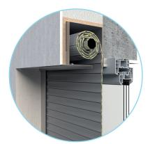
The slats are wound into a built-in box. Part of the box is hardened polystyrene XPS which excels in excellent insulating properties. When the roller shutter is retracted, only the guide rails that are attached to the window frame or to the reveal, the inspection flap and the end slat are visible.
